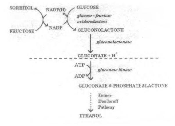
Mechanism of and gluconic acid production by the GFOR and Gl enzymes and gluconic acid conversion to ethanol by the Enter-Doudoroff pathway.
