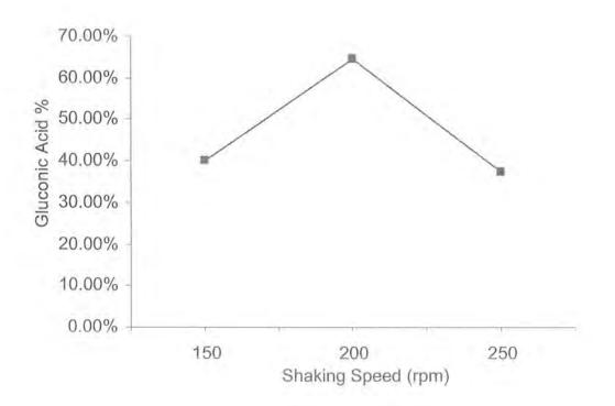
Effect of shaking speed in the presence of MgSO<sub>4</sub> also shows the same results (Table 9, Figure 10). Table 9 shows that at 200 rpm, maximum gluconic acid concentration i.e. 13.14 g/L, percentage was 52.57% and peak area was 551,310. After further increasing the speed at 250 rpm gluconic acid production decreased to 9.60g/L, percentage was 38.44% and peak area was 403,126.
