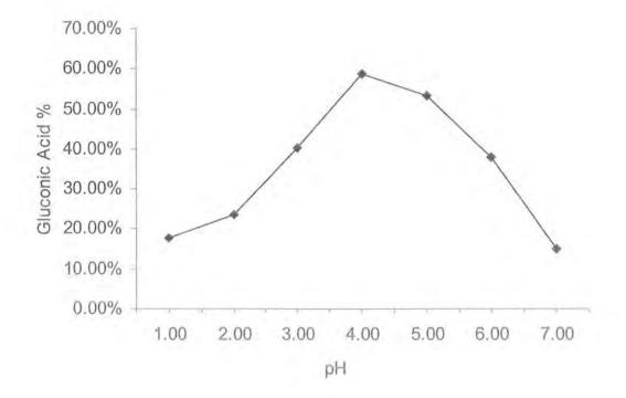
more pronounced and at pH 7.0 the gluconic acid production is only 15.10%, peak area was 158,356 and gluconic acid concentration 3.71 g/L. These all results shown in Table 3 can be seen in a glance in Figure 4.
