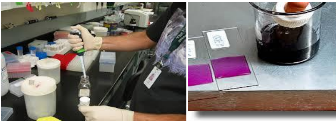
Fig 3.42 a and 3.42 b: Sodium polytungstate (SPT), and acetylated used for the flotation process
