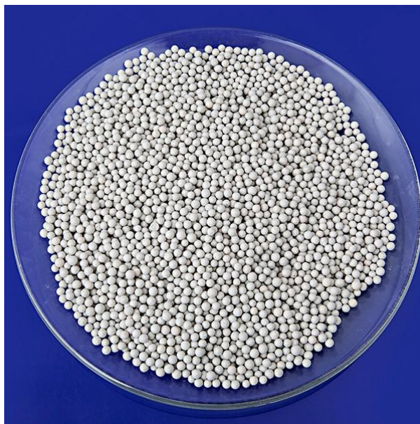
Figure 1: The \gamma\text{-Al}_2\text{O}_3 used as catalyst support
