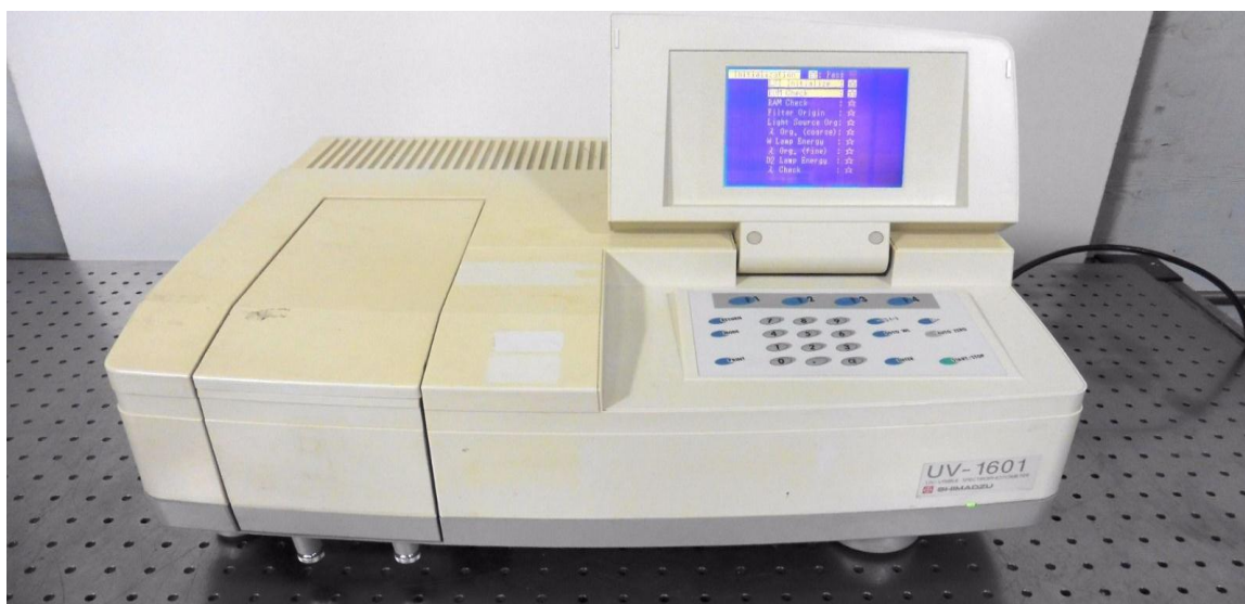
Figure 2.1 UV-Visible Spectrophotometer (Schimadzu 1601)
