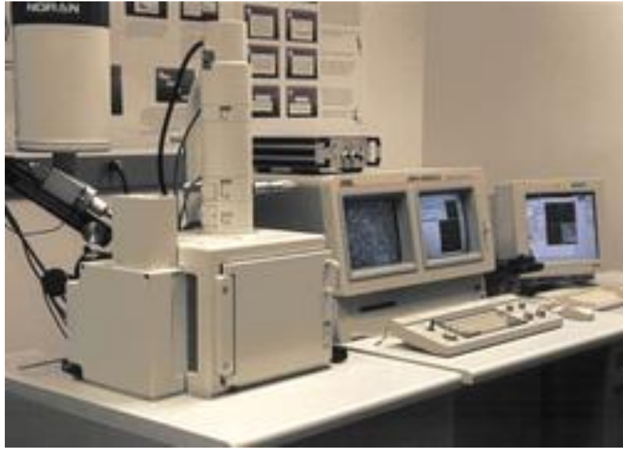
Figure 2.9 A commonly used SEM instrument, with the sample chamber, EDX detector, electron column, electronics console and display monitors.
