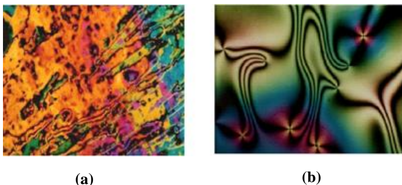
Figure 1.12: (a) Representation of a marble texture for nematic phase in 3-hydroxy-4-(( p -tolyl diazenyl)methyl)phenyl-4-(methylthio)benzoate at 150 °C during heating (b) Schlieren texture for nematic phase in same compound at 234 °C during cooling [41].
