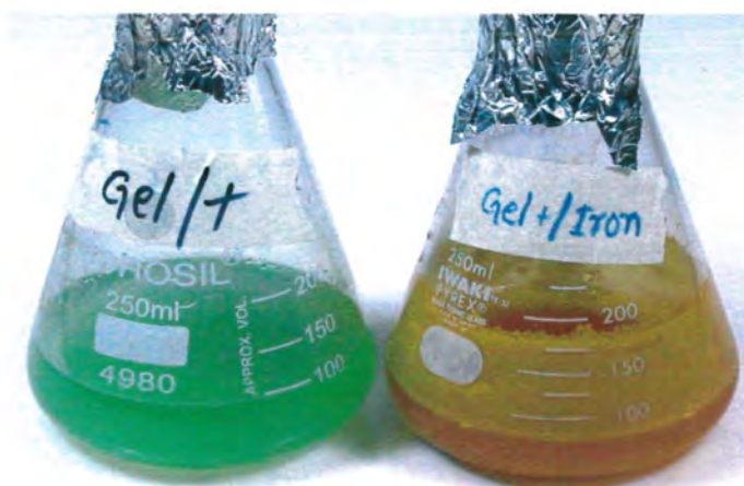
Fig. 11. Conversion of Fe 2+ into Fe 3+ by Acidithiobacillus ferrooxidans at 30 o C, 150 rpm.
