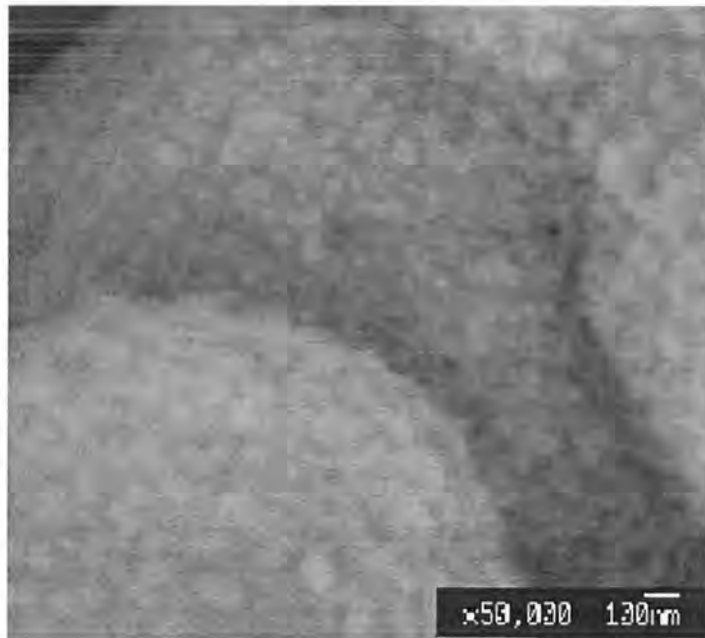
Figure 4.4 \text{TiO}_2 gel particles dried at room temperature
