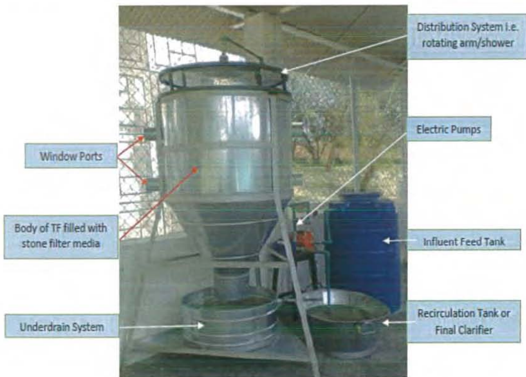
Fig. 3.1 Pilot scale TF system installed in a work station located at the vicinity of the Department of Microbiology, QAU Islamabad for the treatment of wastewater.
