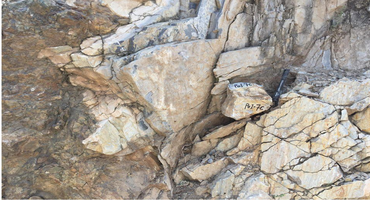
Fig 4.10 Highly fractured limestone, at the contact of the dyke. Dolomitization has occurred along the fractures. Mostly cementing dolomites are present in this sample from petrographic study.
