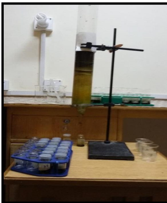
Figure 4.1: Column used for isolation of fractions from the crude extract of G. robusta .
