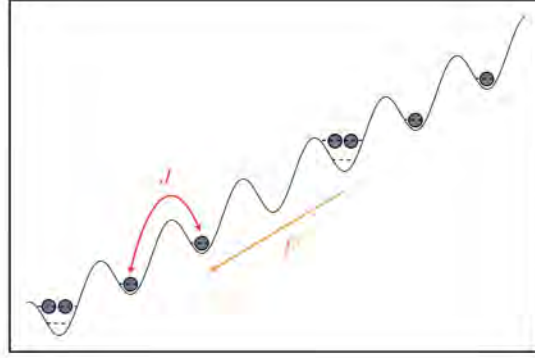
Figure 3.1: Atomic motion in a tilted optical potential. The constant linear force submerged upon the lattice yielding uniform tilt.
