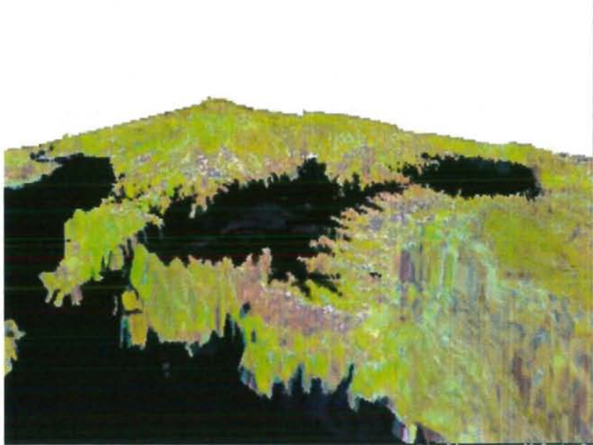
Figure3.11: DTM of the Mangla, Landsat image is overlaid on the DEM of Mangla
