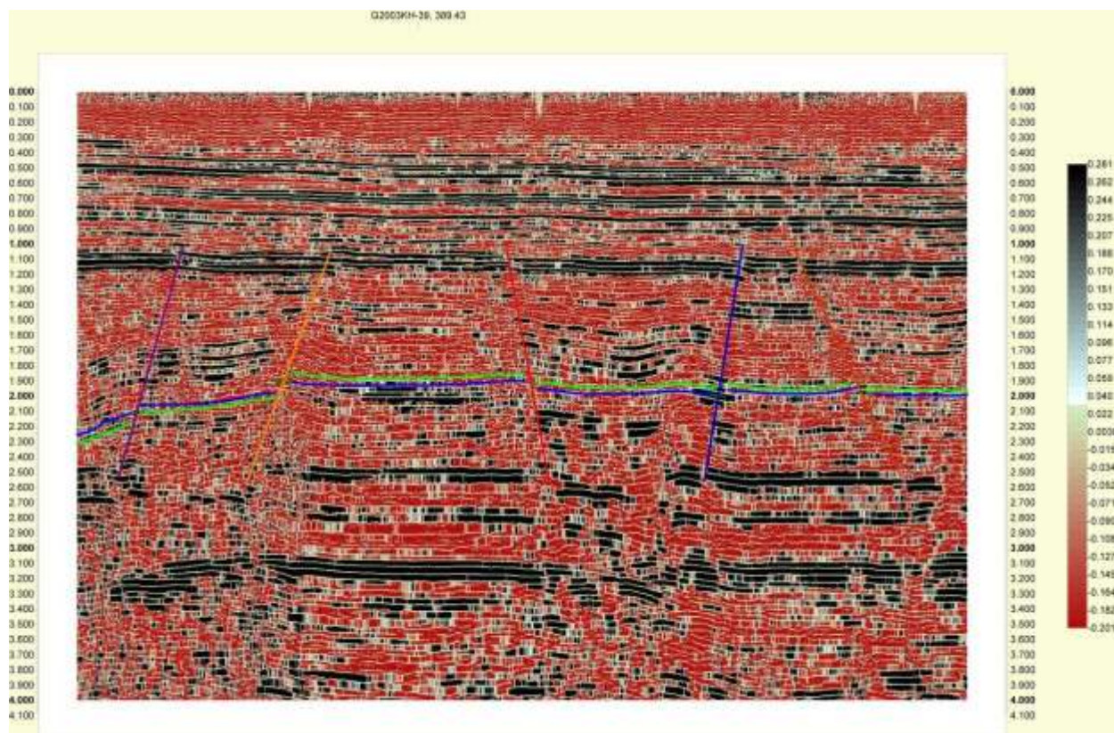
Figure 4.2: Shows the Average Energy attribute applied on seismic line G2000KH-04.
