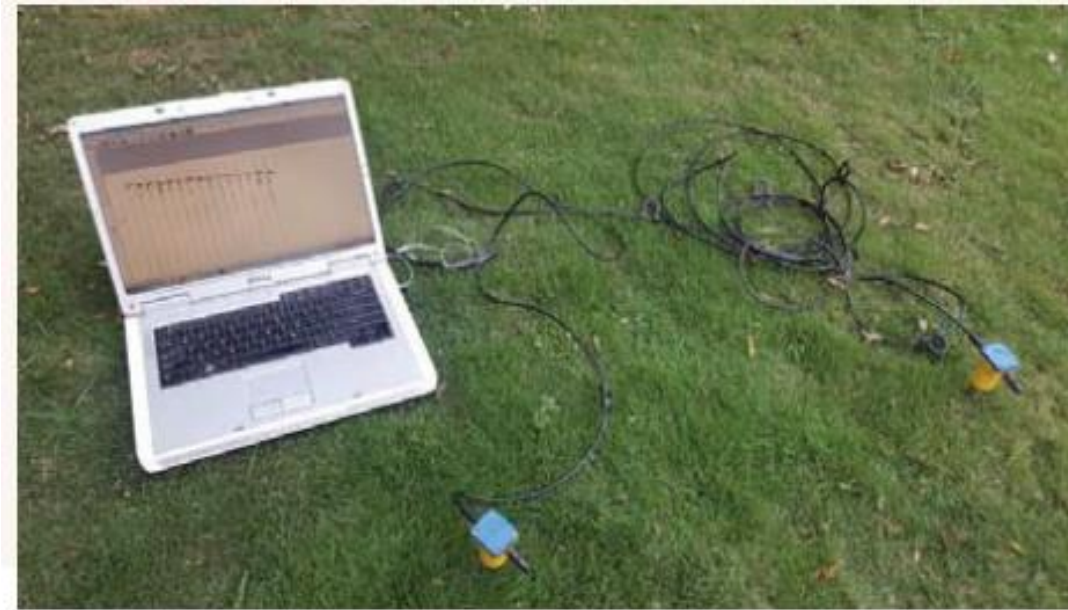
Fig 5.4. Field acquisition with the PC-based two geophone seismic refraction recorder.
