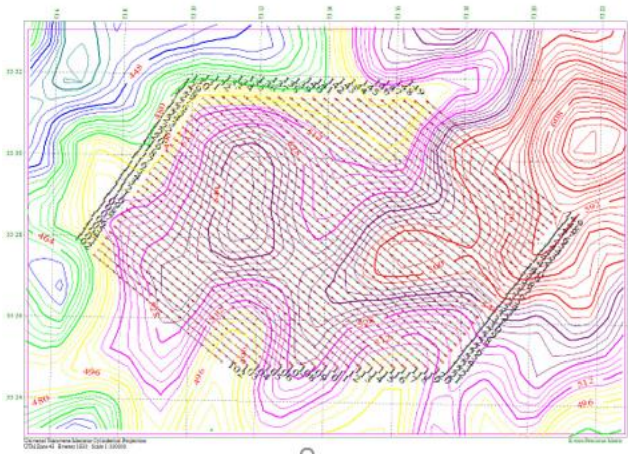
Fig 1.4 SRTM digital elevation model of Study area along with survey grid lines
