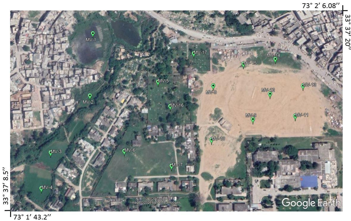
Fig 5.7. Base Map of Survey area for Moisture & Velocity measurement Map shows that data has been acquired at total a of the 17 stations and Moisture & velocity is measured at these stations. Table 5.1 shows the values of measured velocities & moisture percentage at the these stations.
