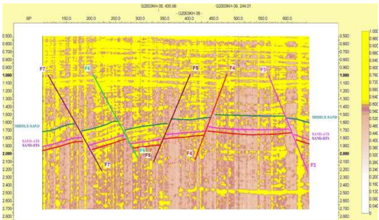
Figure 4.1: Envelope attribute applied on seismic section G2003KH-36, orientation is NE to SW.
