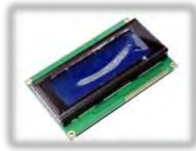
Figure 3.15 20X4 LCD DISPLAY
