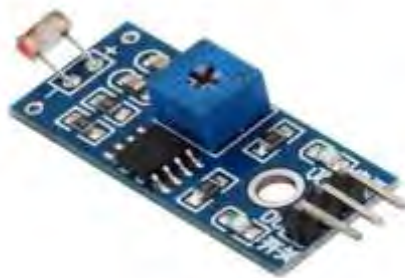
Figure 3.7 LDR Sensor Module
