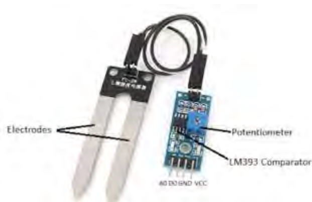
Figure 3.9 Soil Moisture Sensor YL-69
