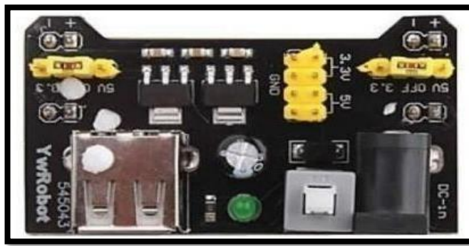
Figure 2.4 Power Supply Board
