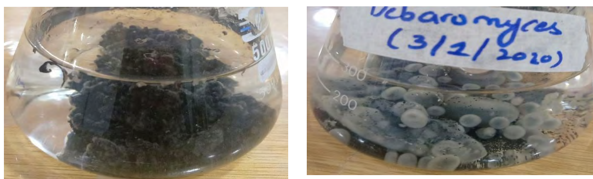
Fig 4.30 Coal Biosolubilization process by potential fungal isolates in Liquid medium using High rank Bituminous Coal
