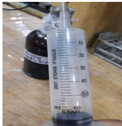
Figure 3.4 Syringe Filled with biogas
