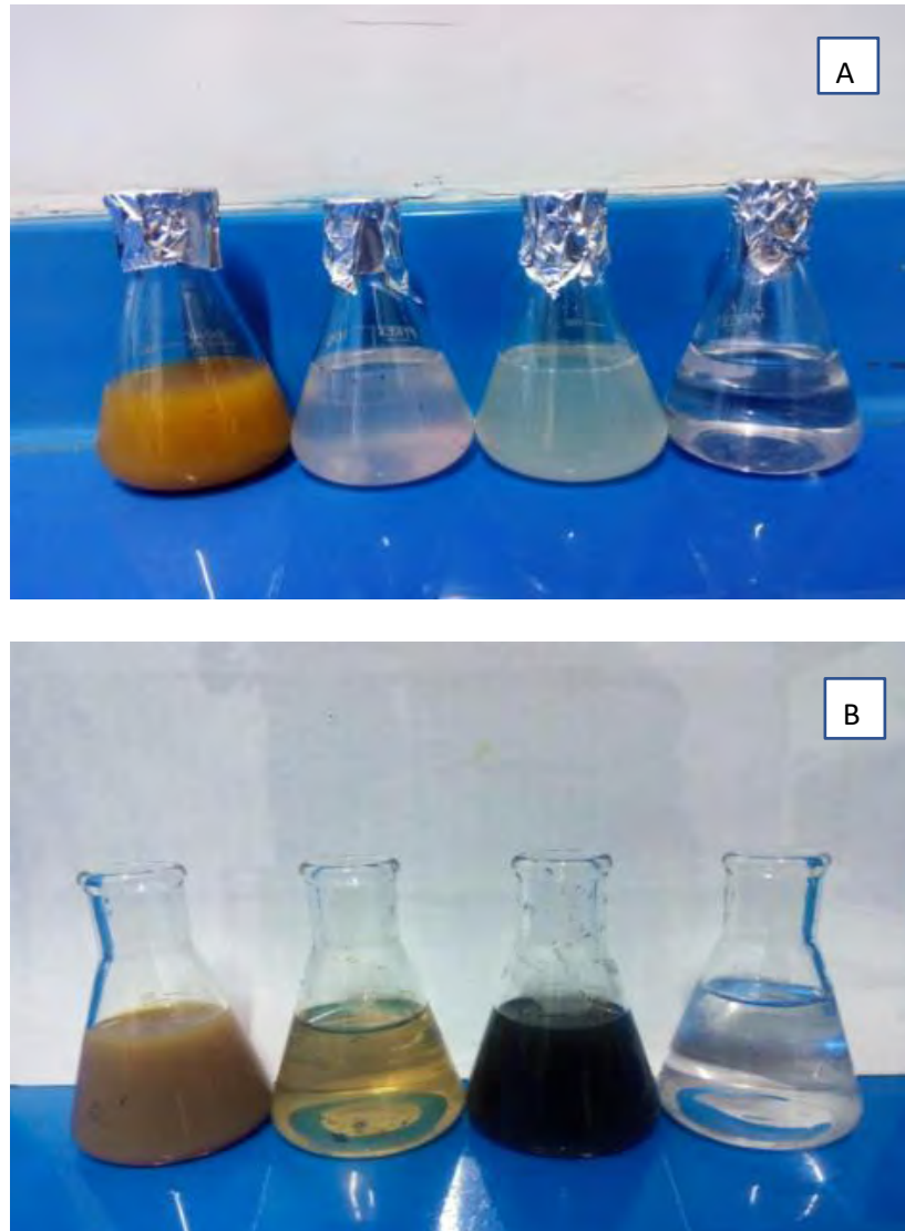
Figure 4.1. Flasks containing bacterial consortium supernatant, fungal supernatant, sugarcane husk extract and distilled water without \text{AgNO}_3 solution (A). Flasks containing bacterial consortium supernatant, fungal supernatant, sugarcane husk extract and distilled water with \text{AgNO}_3 solution (B). Silver nitrate solution without any amendment (negative control), showed no color change when treated with distilled water. However, when silver nitrate was treated with three different samples of aqueous filtrates and supernatant of sugarcane bacteria and fungus, respectively, color of the solution changed to dark brown after 3 days due to the deposition of AgNPs (Fig 4.1).
