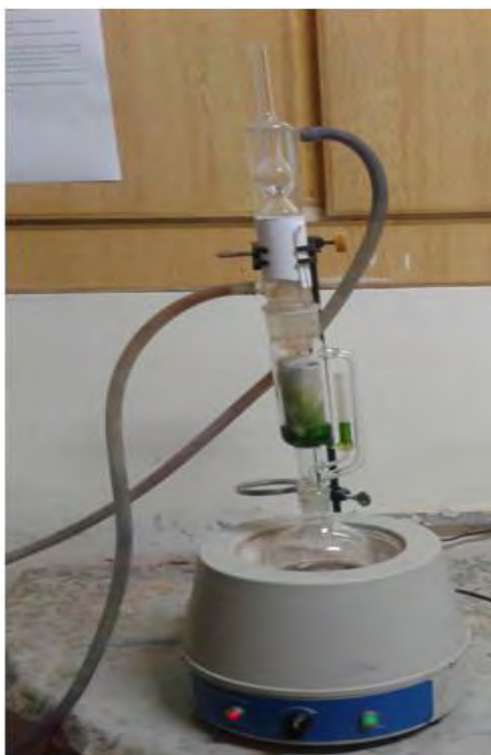
Fig.5.2: P. armeniaca extract preparation in Soxhlet apparatus
