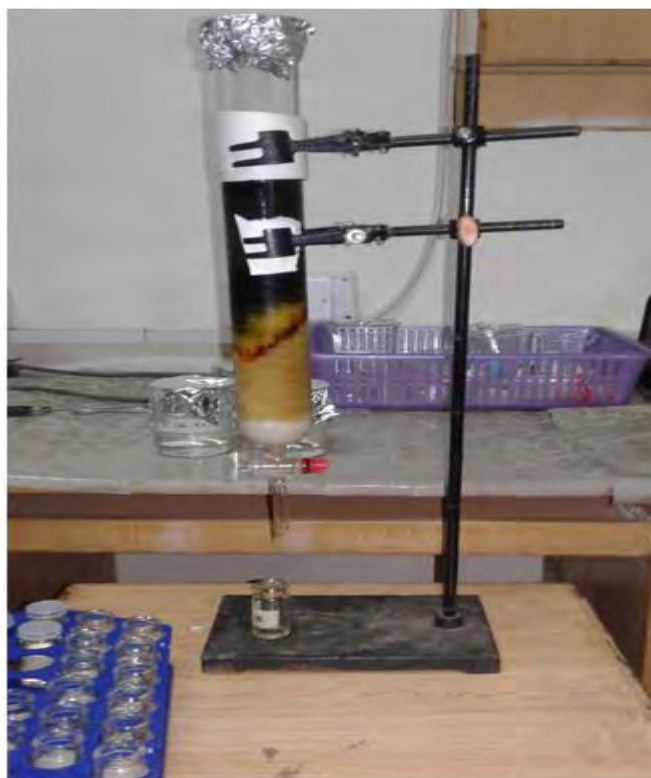
Fig 5.3: Fraction isolation by column chromatogragy
