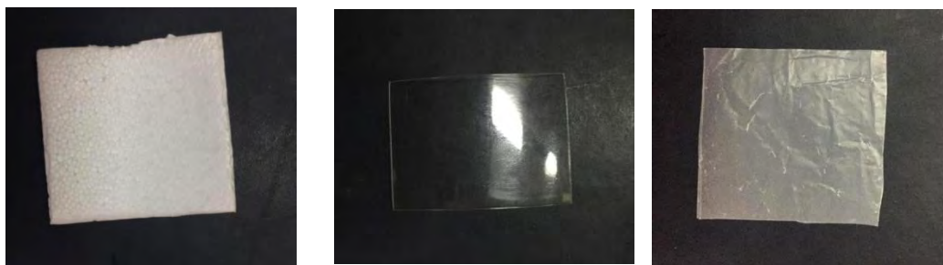
Figure 9: Weighed and Equal Size Strips of PE, PS, PET used for degradation
