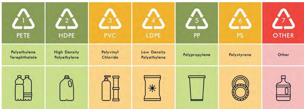
Figure 1.2 Symbols and codes of seven plastic types
