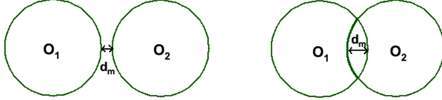
Figure 4.3: Positive and a negative distance of minimum approach d_m between two ideal track circles
