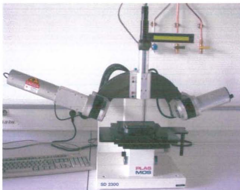
Figure 2.7: Photographic image of the PLASMOS SD-2300 ellipsometer.
