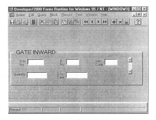
This form contains information about the items, along with other necessary information, which have passed through the gate by any mean. Here B\_No and Item\_code are the foreign keys.
