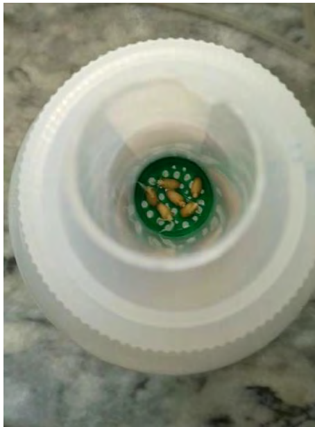
Figure 2: Falcon tubes containing seeds, fixed into the bottle
