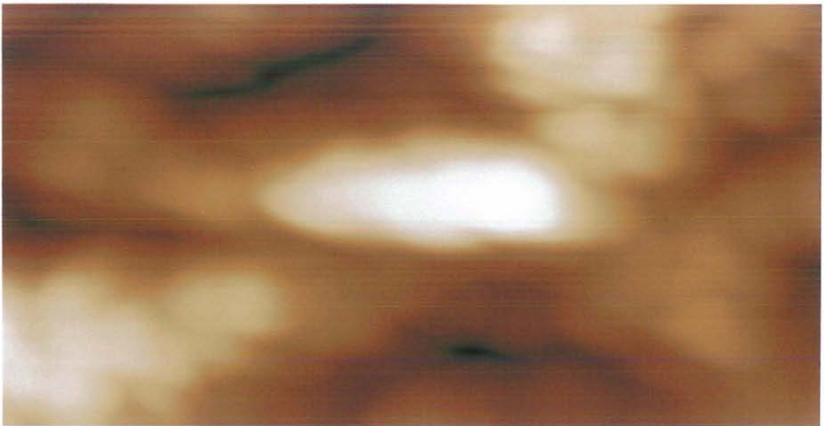
Fig. 4.3f 2-D AFM image of PbO 2 electrodeposited on Pd substrate with an area of 2 μm × 2 μm.
