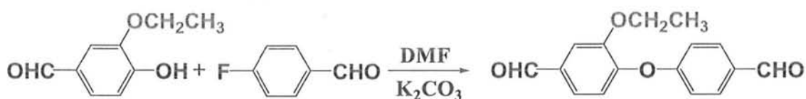
2-ethoxy-4,4'-diformyldiphenyl ether (EDF)
