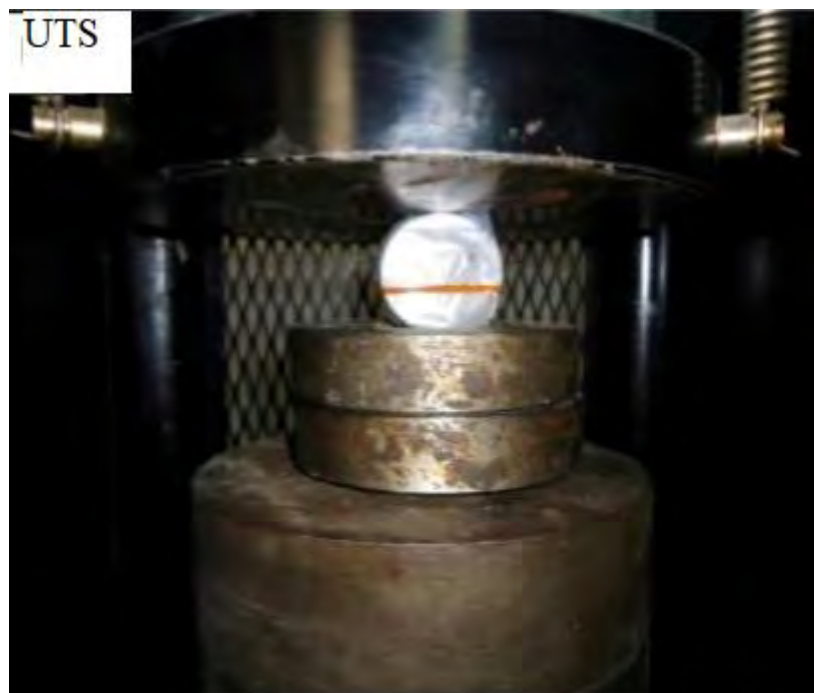
Fig. 5.1. Universal testing machine (UTM), sample for UCS test and Universal testing machine (UTM), sample for UTS test
