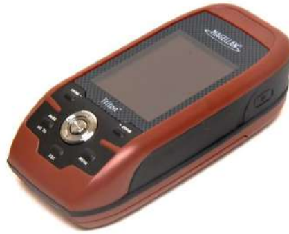
Figure 4.2 Magellan Triton 400 handheld GPS on which coordinates were stored and utilized in navigation towards the survey points.
