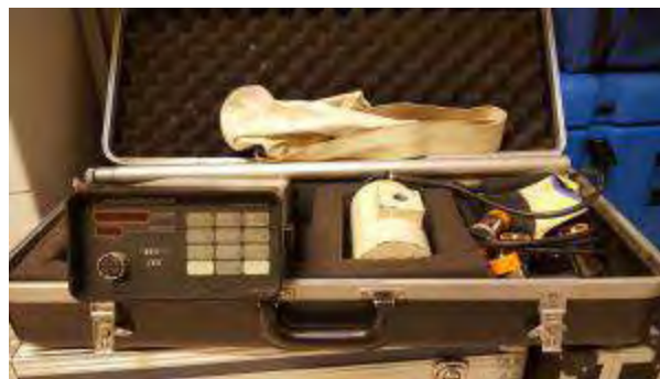
Figure 4.3 Geometrics G-856 Proton Precision Magnetometer which was used to acquire field data.
