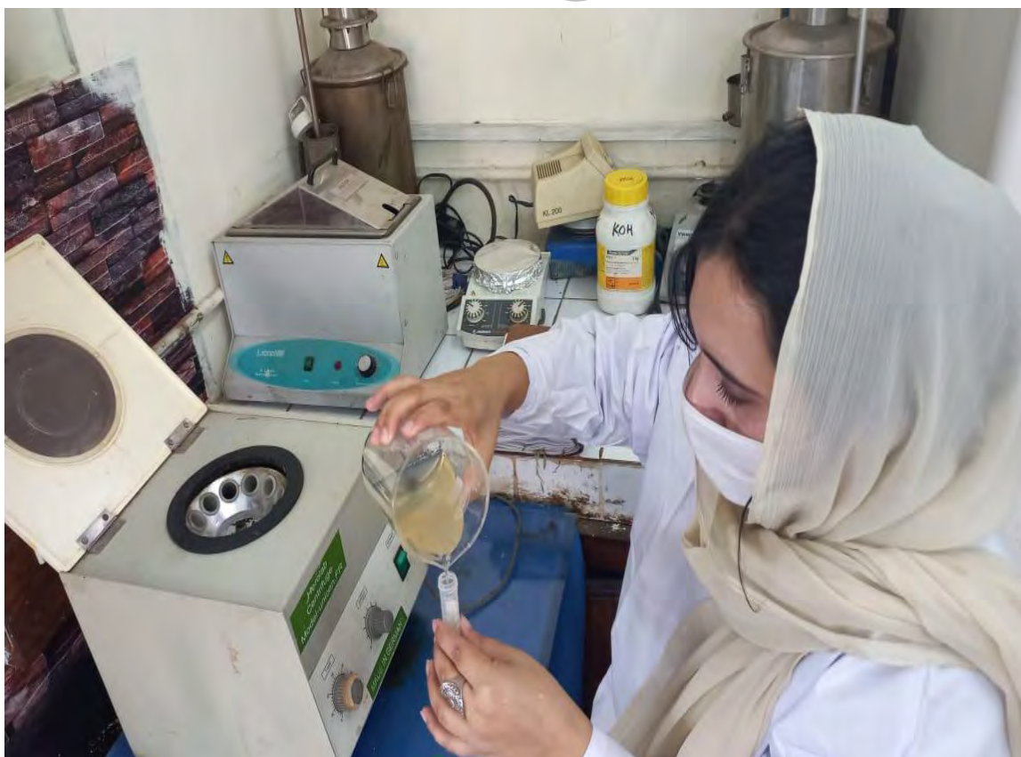
Plate 13. Honey analysis experimentation (A) Honey samples in beaker string at hot plate species (B) Poured honey sample into falcon tube for centrifugation
