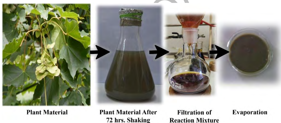
Figure 3.7. A generalized illustration of crude extracts preparation. It involves soaking plant material into the solvent of the desired polarity, followed by shaking for 72 hrs, filtration, and evaporation of filtrate.
