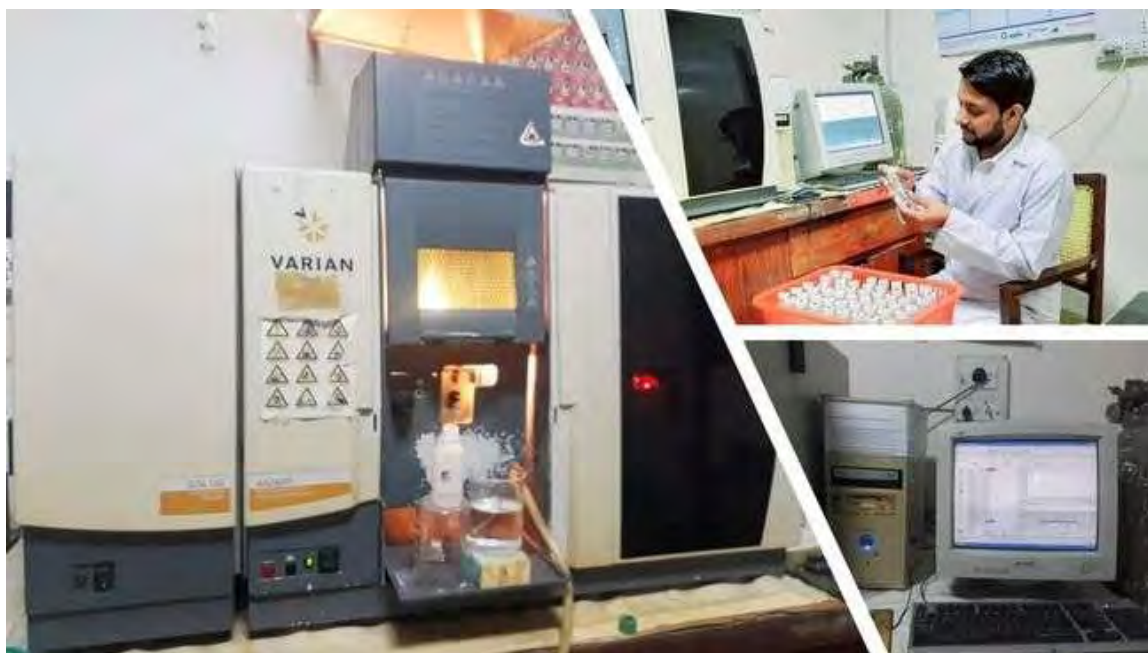
Fig. 4.4 Quantification of PTEs using atomic absorption spectrophotometer.
