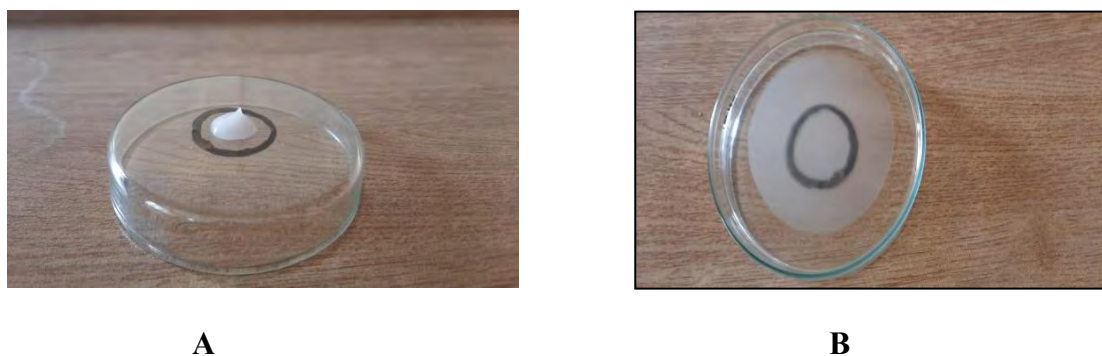
Figure 3.14. A and B shows spreadability of MCZN TESSs gel via glass slide method.
