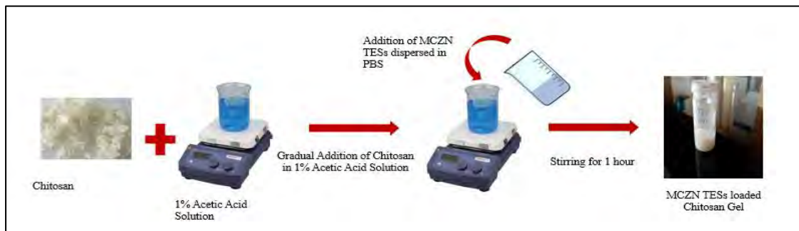
Figure 2.2. Method of preparation of chitosan gel.
