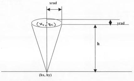
xc,yc = center coordinates h = heightxrad = semi-major axis of base yrad = semi-minor axis of base yrad = 1/3 xrad
