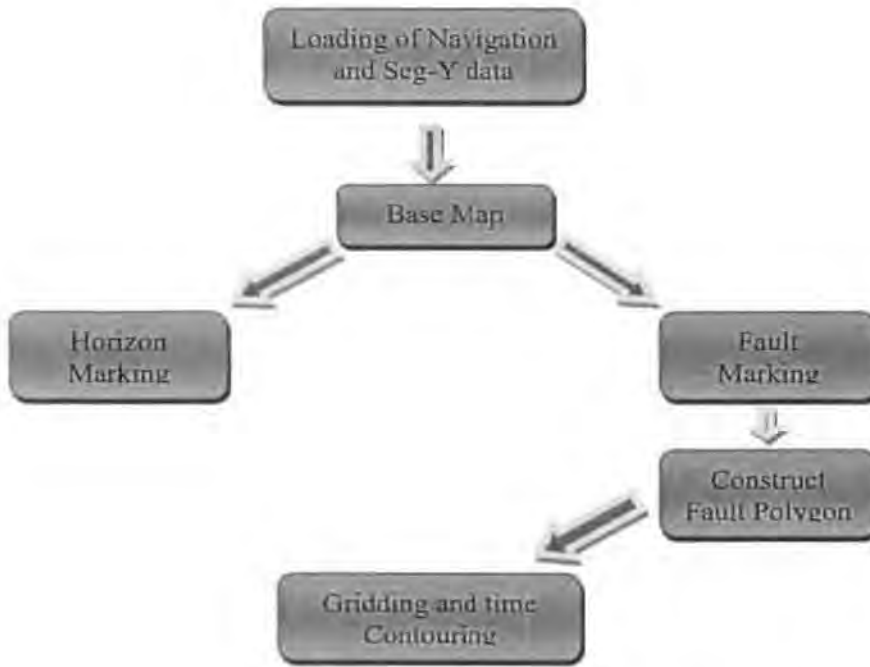
Figure 4.1 Work flow for seismic data interpretation
