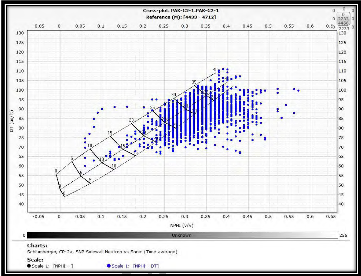
Figure 5.5. Neutron-density cross plot for lithology and minerals identification (Schlumberger log interpretation charts, 1997).
