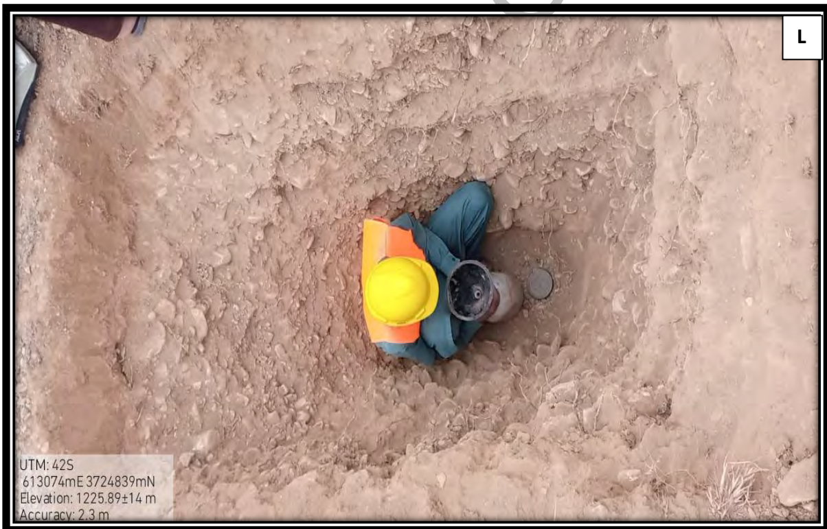
Figure: 3.11:- Photographs showing test pits progress. (K) Measuring the specific advised size of a standard test pit at the site. (L) The process of performing F.D.T in the field.
