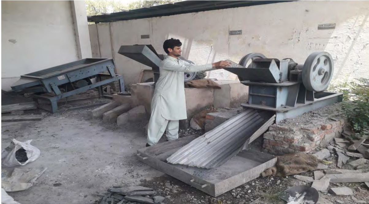
Fig: 3.2 Blake Jaw Crusher machine at PCSIR lab Peshawar.
