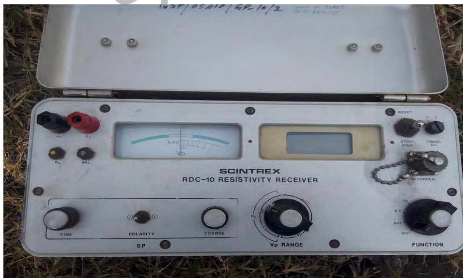
Fig. 3.8: RDC-10 Scintrex Resistivity Receiver is used to calculate the value of resistivity during resistivity data acquisition.
