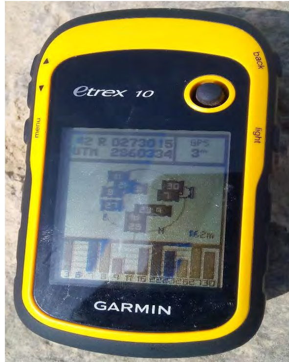
Fig. 3.4: Garmin hand-held GPS used to determine the coordinates of the observation stations.
