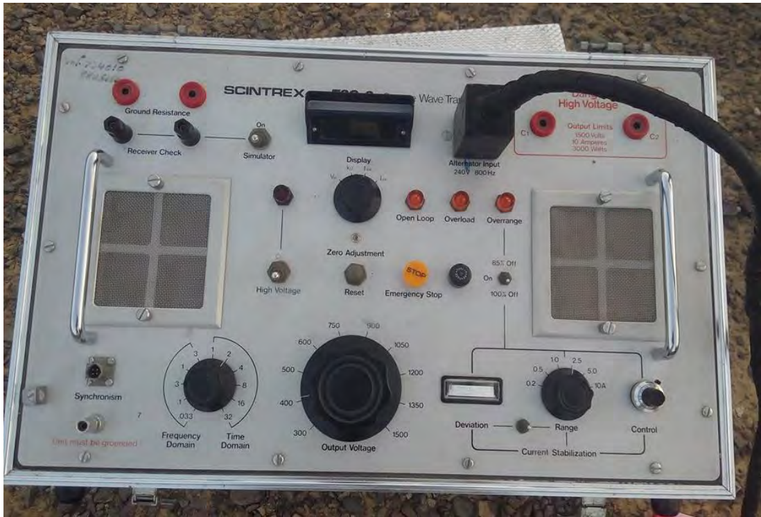
Fig. 3.6: TSQ-3 Scintrex Resistivity Transmitter is used to control transmission of electric current to current electrodes during resistivity/IP data acquisition.
