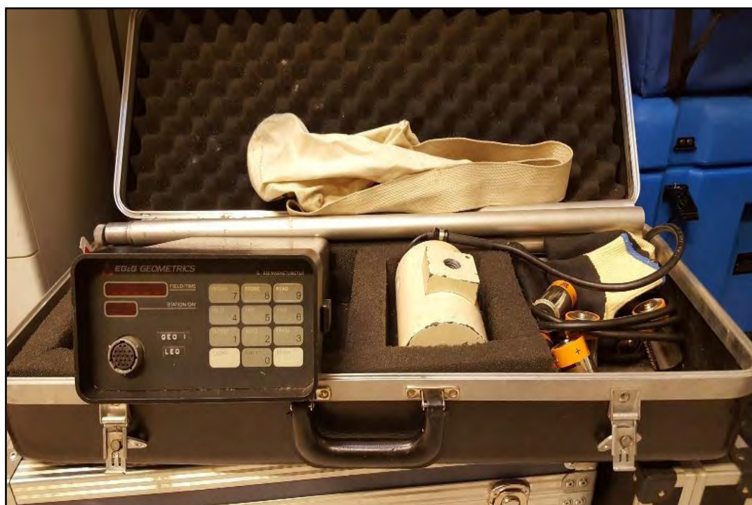
Fig. 3.3: G-856 Geometrics Proton Precision Magnetometer used for magnetic data acquisition.
