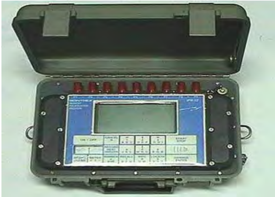
Fig. 3.7: IPR-12 Scintrex IP/Resistivity Receiver is used to calculate the value of chargeability and resistivity during resistivity/IP data acquisition.
