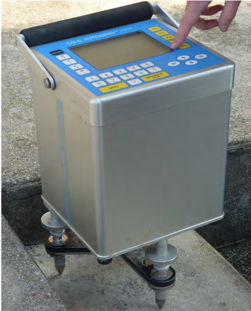
Fig. 3.5: CG-5 Scintrex Autograv gravimeter used for the gravity data acquisition.
