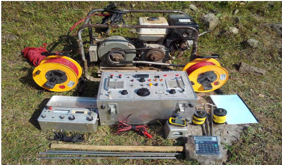
Fig. 3.9: Resistivity Generator along with all necessary instruments used for carrying out the resistivity/IP data acquisition profiles.
