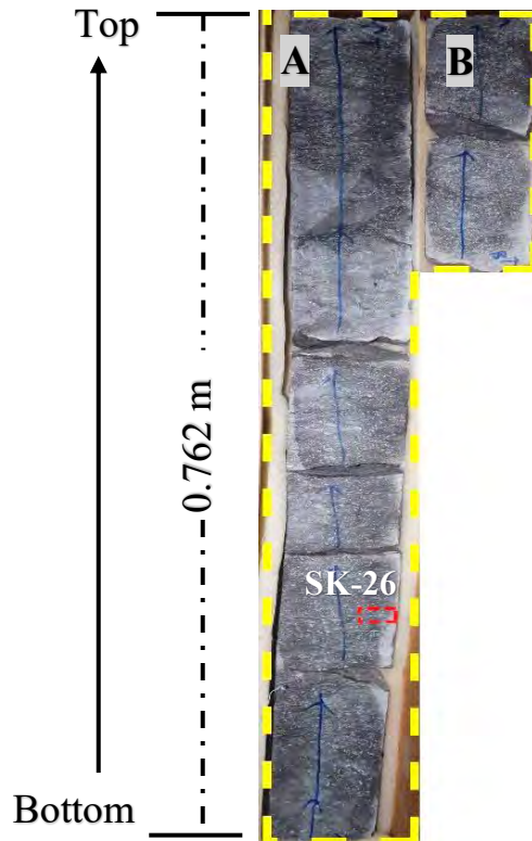
Figure 4.12 Photograph showing core slabs of core-45, labeled A-B represents the top and bottom part of the core slabs respectively, dotted yellow lines marked the different intervals and dotted red lines are the sample locations (SK-26).
