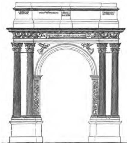
FIG. 2.—OPENING SPANNED BY A SEMICIRCULAR ARCH. ROMAN TRIUMPHAL ARCH AT POLA.
