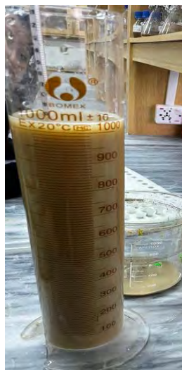
Figure 15: Using Hydrometer to Find Soil Texture
