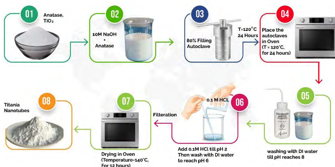
Figure 2.1: Synthesis scheme of titania nanotubes
