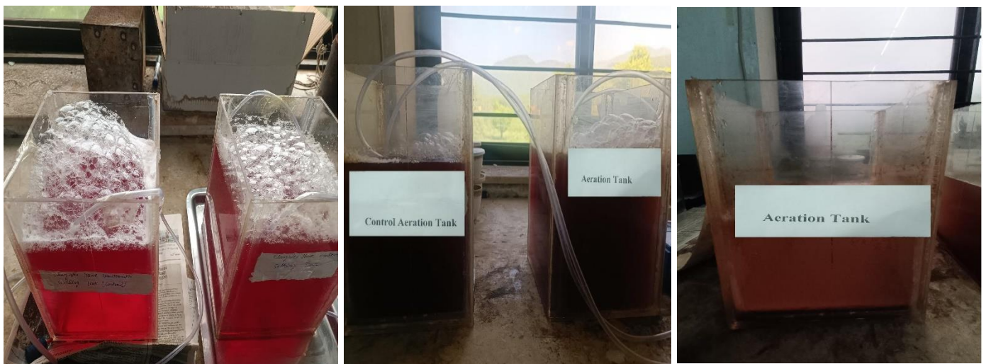
Aeration treatment of abattoir's wastewater
