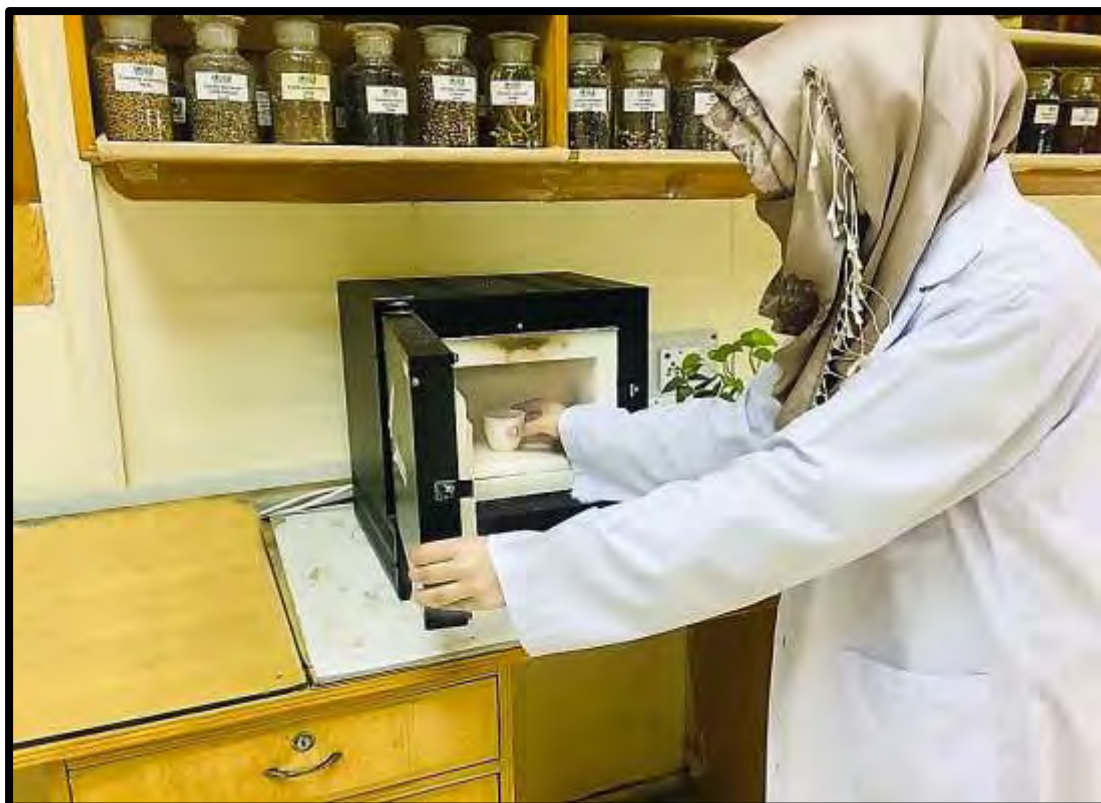
Plate 14 Calcination in Muffle Furnace
