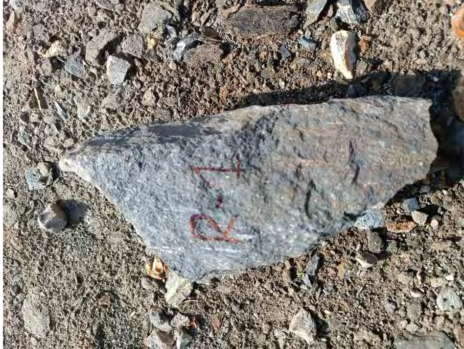
Figure 3.1: Site Photographs: Medium grade Schist rock.
