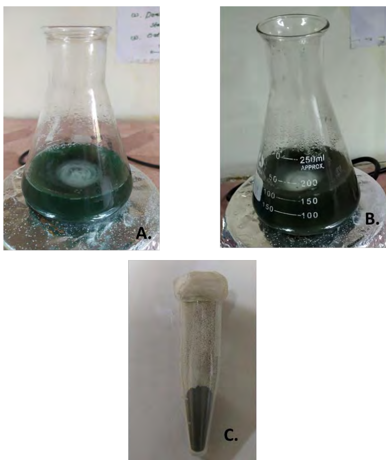
Figure 4.1: Colour change shows synthesis of CuO-NPs. A. Green coloured extract. B. Dark brown coloured extract. C. Powdered CuO-NPs after incubation and calcination
