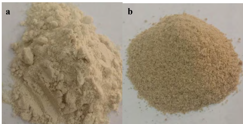
Figure 2.2: Treated and untreated samples (a) Untreated industrial gluten (b) After enzymatic treatment
