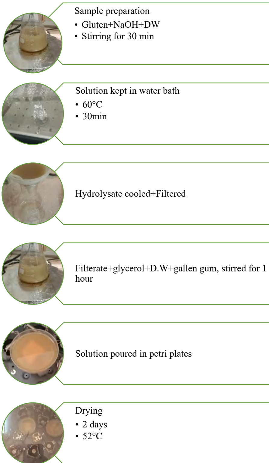
Figure 2.7: Schematic representation of film preparation
