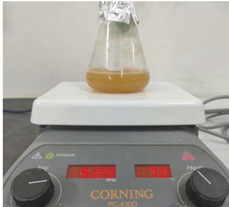
Figure 2.8. Magnetic stirring of sample Treating the fibers with sodium hydroxide and nitric acid at 70 °C on magnetic stirrer for 10h.
